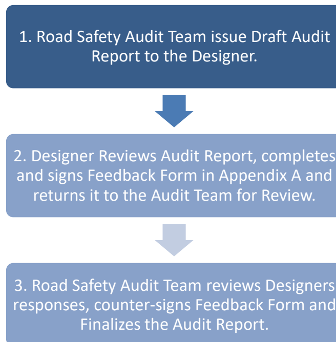
Figure 5.1 – Road Safety Audit Sign-Off and Completion Process
