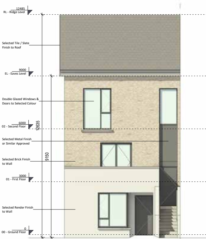
① Front Elevation 1 : 100
