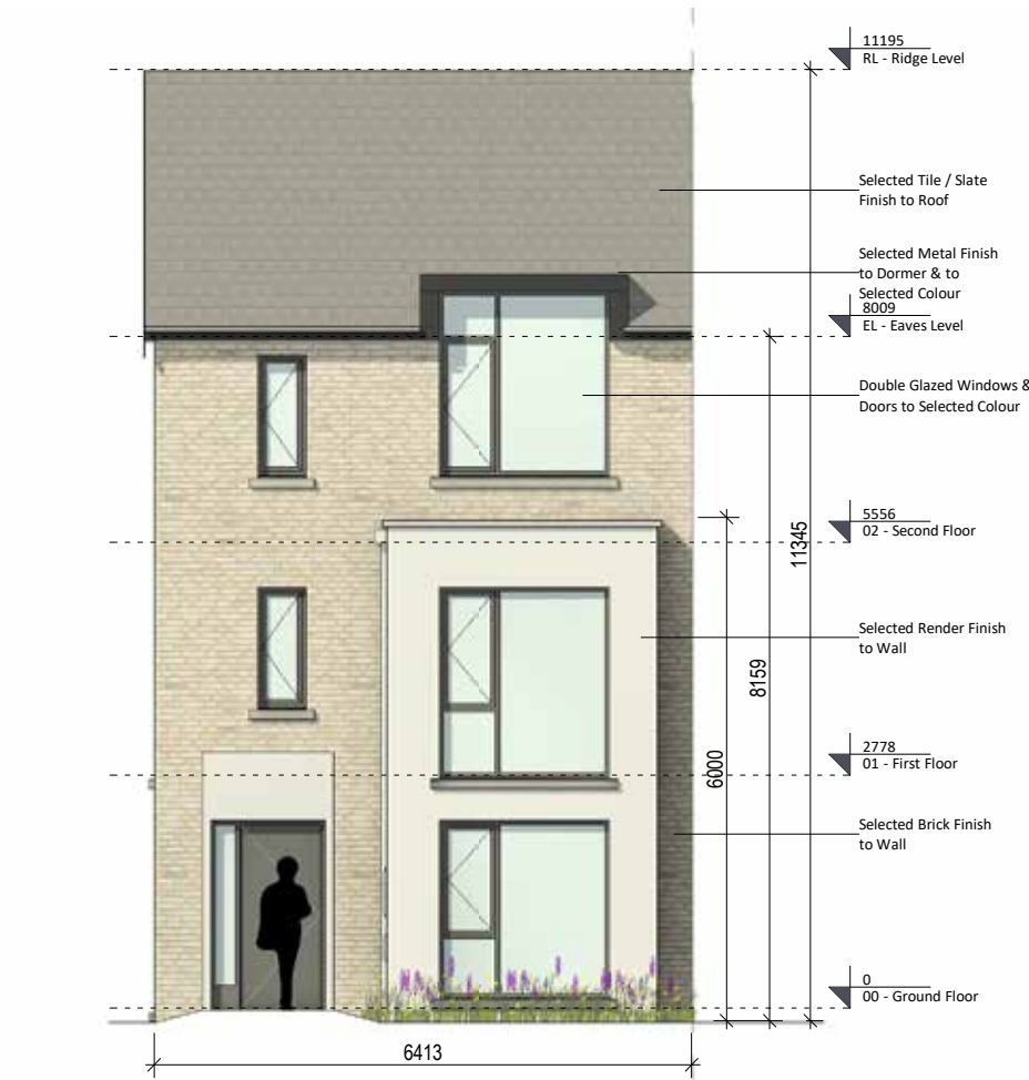
④ Front Elevation 1 : 100
