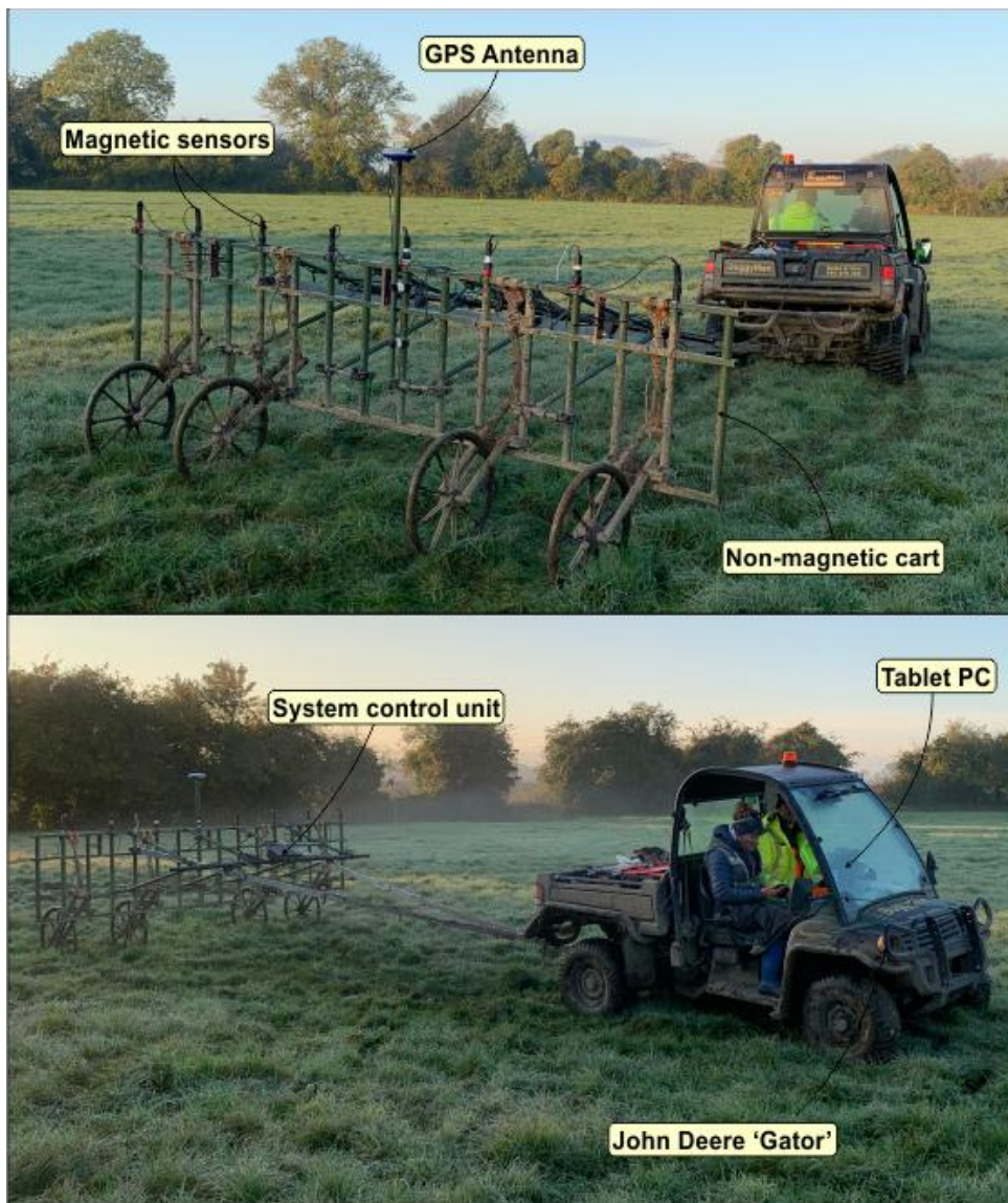
Plate 4: John Deer Gator and Sensys Magneto MXV3 (Library photo).
