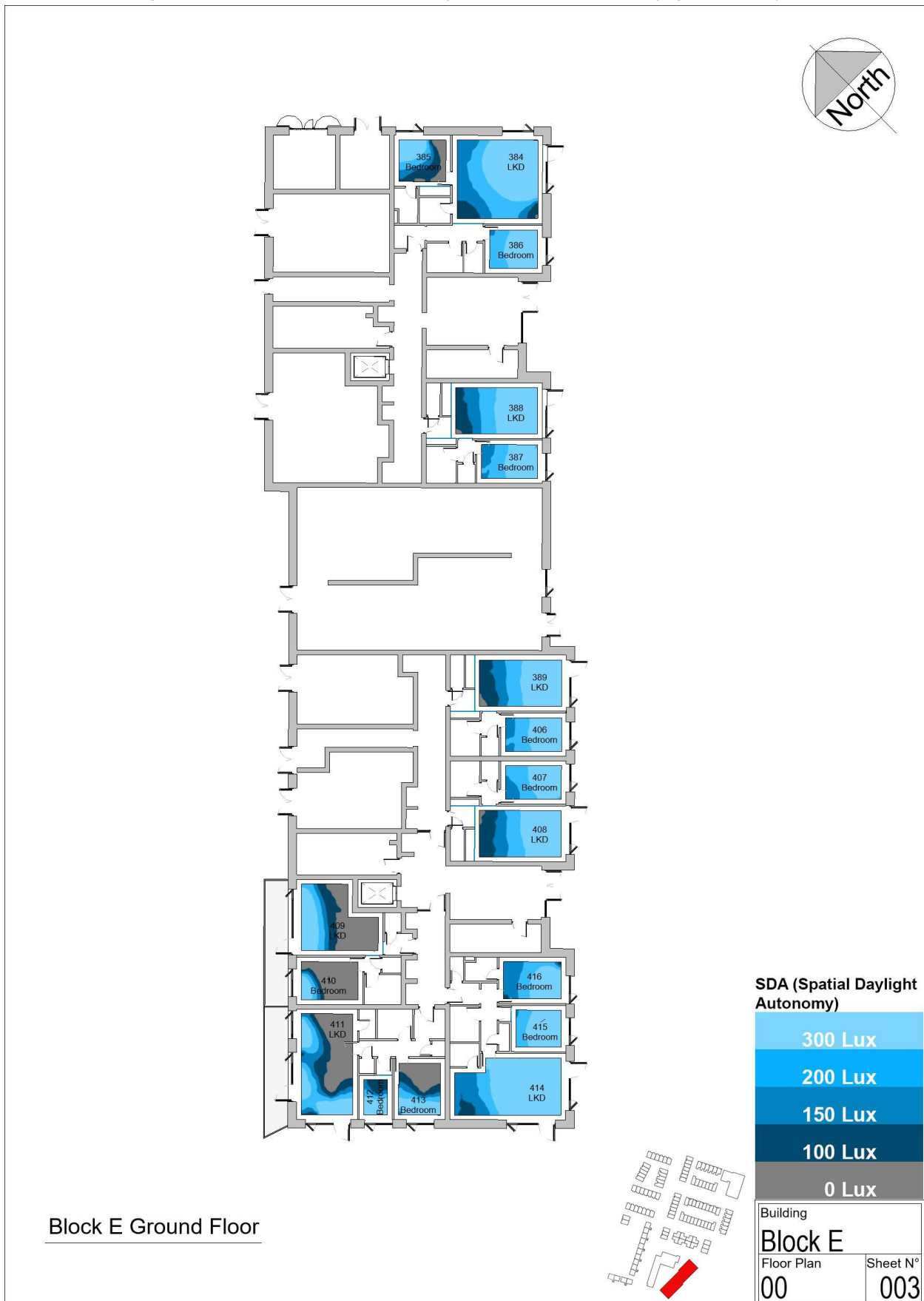
Figure 6 - Block E Plans with Room Reference Numbers and Daylight Heatmaps
