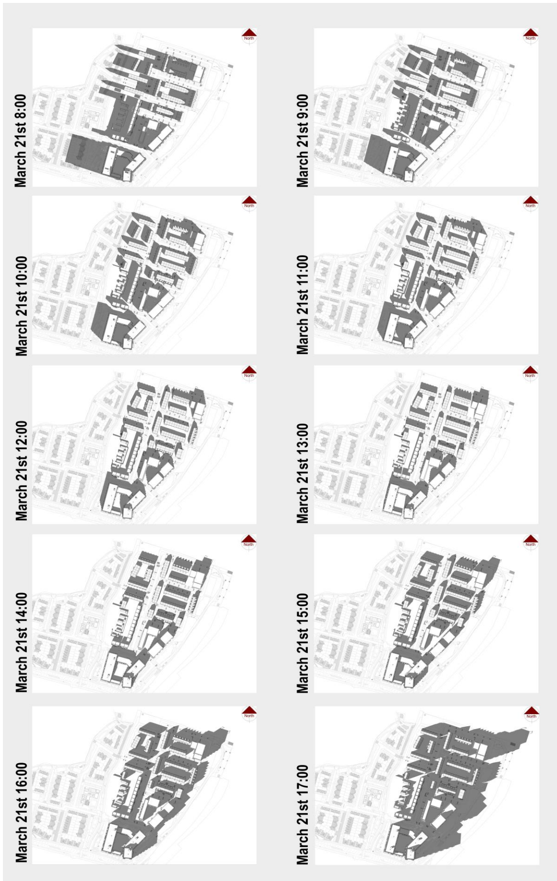
Figure 10 Shadow Diagrams - March 21 st Spring Equinox
