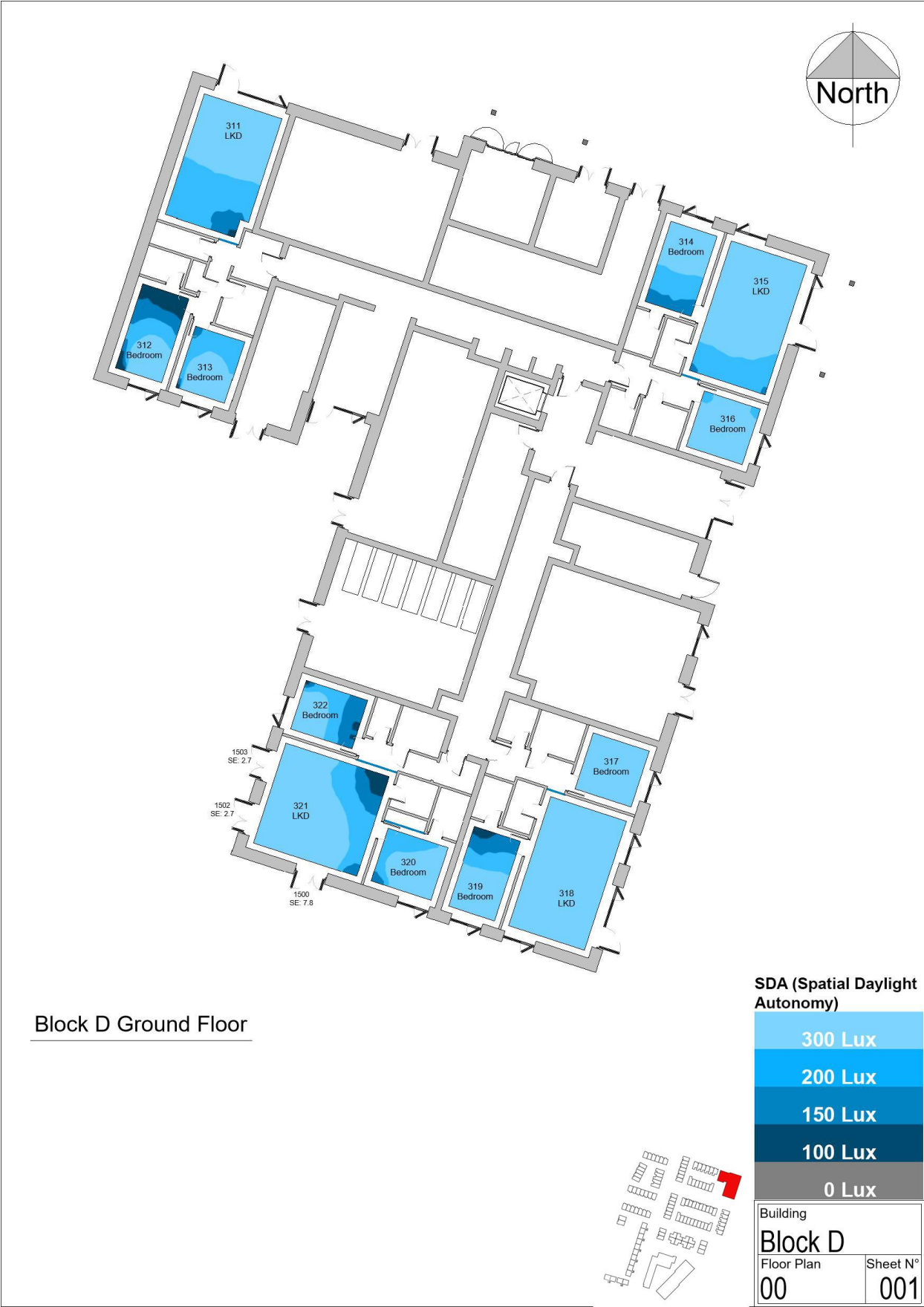
Figure 5 - Block D Plans with Room Reference Numbers and Daylight Heatmap
